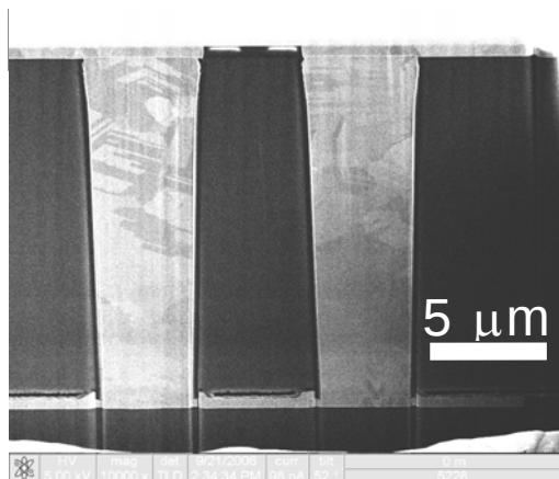
Fig. 11: Through-Si vias realized at IMEC (left) and advanced 3D-stacked imager concept (right). Multiple layers of circuitry (digital and analog) as well as micro-optics will render a highly efficient system-on-chip (SOC) solution for imaging
